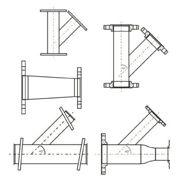
Reasons for S10 fittings w/ 150# flanges: price press rating of S10 sometimes higher than flange rating Reasons for S40 fittings w/ 150# flanges: corrosion factors strength erosion factors
