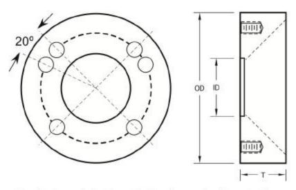
Transmitter flanges allow for the mounting of sensitive measuring devices onto tanks. The offset bolt pattern accommodates a transmitter isolation valve or direct mount of a level transmitter.
